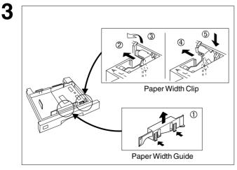
Adjust the Paper Width Guide and Clip to the proper paper (A4, or LTR/LGL).
